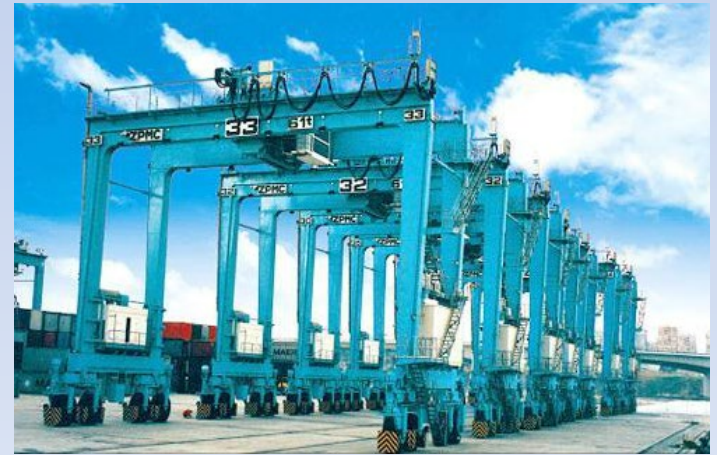
Rubber Tyred Gantry Crane
